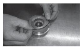
14. Then, remove the stationary seal which has been fitted into the cover.
