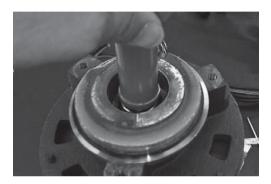
5. Install the key into the key way of the motor shaft.
