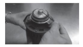
6. Move the impeller forward together with the cover (back casing).
