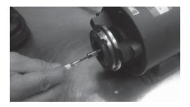
10. Move the dynamic seal from pump, together with the cover (back casing).
