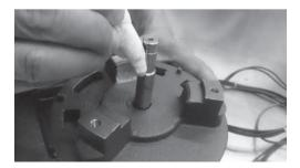
3. Clean the outer surface and step part of the motor shaft.
