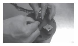
2. Install a new stationary seal into the cover.
