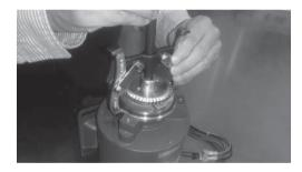
7. Remove the impeller by hand.
