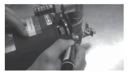
3. Loosen the hexagon socket head cap screws that have fixed the body.
