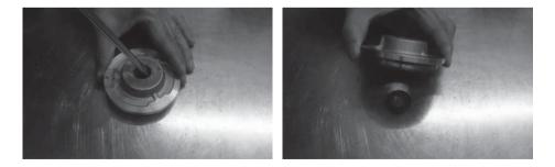
15. Pull the rubber washer off of the motor shaft.
