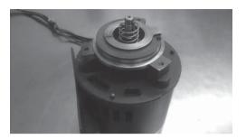
7. Install the impeller onto the motor shaft.
