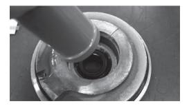
3. Install the cover with the stationary seal onto the motor shaft, and push it into the motor bracket.
